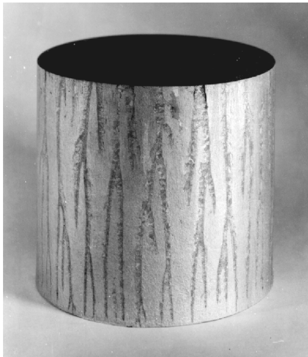
Directionally Solidified Superalloy Ingot (A. F. Giamei, UTRC)
